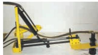
It's powered by tractor hydraulics and will trim a 24-in. dia. circle.
