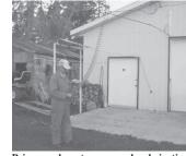
Primrose also set up an overhead pivoting air hose, which swings out 15 ft. from the outer wall of his shop.
