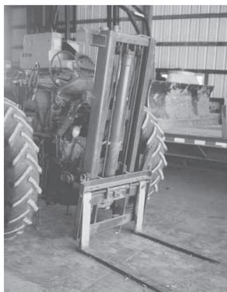
Noel Hicks "modernized" his Farmall M by equipping it with live hydraulics and a forklift mast on back. "It can lift 3,000 lbs. up to 8 ft. high with no problem," he says.
