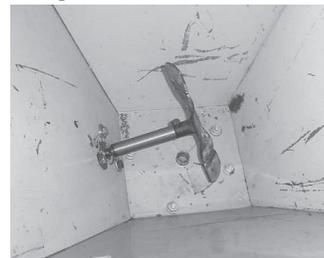
Impeller rotates at 400 rpm's and is hooked into utility vehicle's 12-volt system. To make the impeller he heated up an 8-in. length of flat metal and twisted it, then welded it onto a shaft on the wiper motor.
