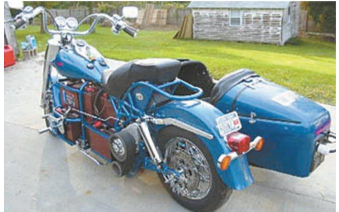
Carl Vogel's 78 hp motorcycle is electric-powered by 10 Trojan 12-volt batteries.
