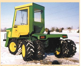
Front tractor is a Deere 318 model, and the back is a 317. Tractor's eight wheels are off the original garden tractors.
