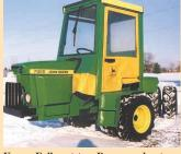
Kenny Fulk put two Deere garden tractors together to build this 1/4-scale Deere 7020, 4-WD articulated tractor.
