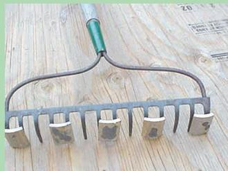
Cleaning up spilled or dropped nails is a good use for rare earth magnets. By attaching them to rake fingers, you can sweep through gravel to remove any fallen nails.
