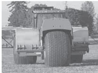
Tractor's front axle is replaced by a front fork assembly and a large single floatation wheel.
