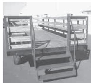
Wagon has three steel steps with hand rails on back. Bottom step is hinged and can be folded up out of the way.
