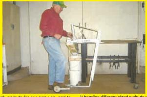
I crack walnuts for our own use, and to give to friends. I built the machine out of material I had on hand such as angle iron, square tubing and wheels from an old lawn mower. The unit is controlled by a foot pedal on wheels that can be repositioned to adjust the leverage.
