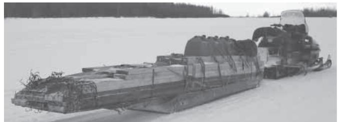
UHMW poly stays flexible at temperatures down to 60 degrees below zero.
