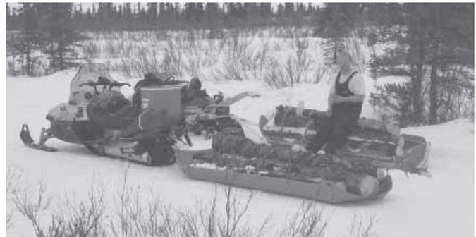
Sleds made from 1/4-in. UHMW poly come with triangular tongues for pulling behind snowmobiles, ATV's and other machines.
