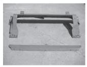
Upgraded feeder house tilt frame for Deere Contour Master combines.
