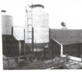
I made a 2-ton bulk feed bin by mounting a 1-ton hog feeder upside down on top of an identical feeder and bolting the two together. I used channel iron to build 8-ft. long legs that bolt to the bottom feeder. Angle iron was also used to build a ladder that extends to the top of the bin where I made a fill hole by cutting off the bottom of the top feeder and hinging one side. (Roger Fisher, Box 9048, Spirit Lake, lowa 51360)
