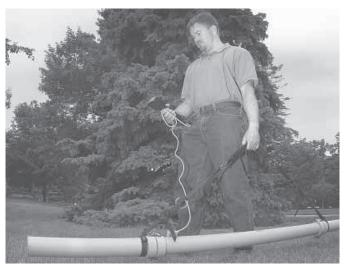
Hand held data reader is connected to sensors inside an 8-ft. long pipe. It works because soil contaminated with household waste has a higher electrical conductivity.
