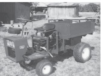
"It's a nice little vehicle for yard work," says Roy Gray, about the electric lift dump truck he built out of a 1960's Allis Chalmers 616 garden tractor.
