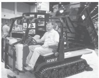
The new ASV Scout, with its 4,000-lb. bed capacity and 5,000-lb. towing capacity, is designed for much heavier work than most utility vehicles.
