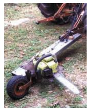
A hand-operated lever is used to swivel the chainsaw and the plate against tree trunks.
