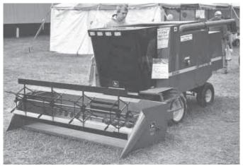
Kenny Fulk turned a pair of Cushman front deck riding mowers into a 5-ft. tall, 6-ft. wide replica of a Deere 9500 combine. Some of the harvest parts actually work.
