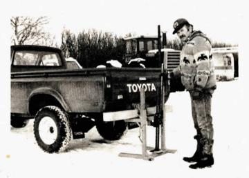
Once up, the Safe Jack holds its position so the lifting jack can be moved to another location.
