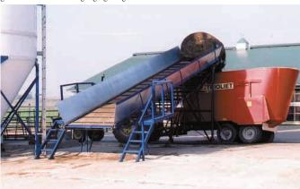
Home-built 30-ft. long, 12-ft. high elevator is used to load silage bales into Clavin's tub
