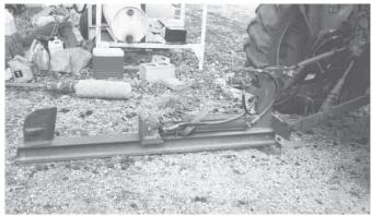
Home-built, 3-pt. mounted log splitter uses an old railroad rail as the main beam.
