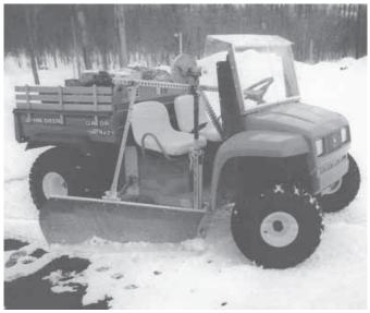
Side-mounted blade is operated by two hand controls, both located at floor level in front of passenger seat. Home-built plastic windshield extends over the dash.
