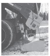
Material is augered into bottomless threesided box, which hangs from back end of gravel truck.
