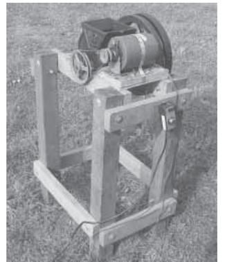
Apple grinder's drum is belt-driven by an electric motor.
