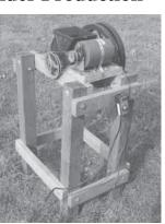
Apple grinder's drum is belt-driven by an electric motor.
