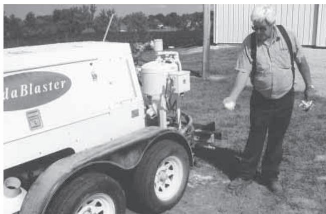
**Charles Klein with a handful of soda that he uses with his trailer-mounted “Soda Blaster” cleaning machine. Unit cleans with baking soda instead of sand.**
