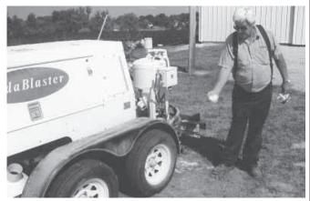
Charles Klein with a handful of soda that he uses with his trailer-mounted "Soda Blaster" cleaning machine. Unit cleans with baking soda instead of sand.
