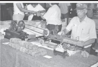
Carl Veldhuizen makes small bales using a mini stationary baler that's powered by a model "hit and miss" gas engine that he put together from a kit.
