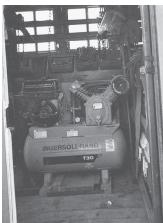
Front part of trailer contains a 25 cfm, gaspowered air compressor and generator.
