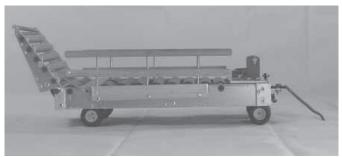
The SMART cart has a 3-ft. end gate that drops down hydraulically to the ground.
