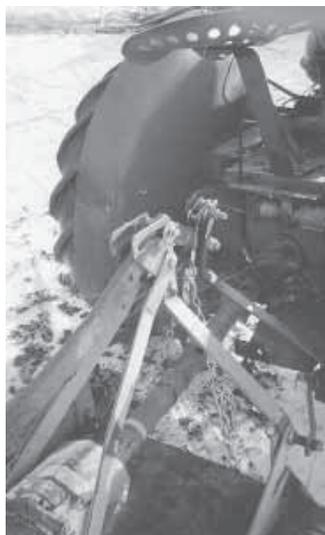
**A 12-volt, 1,000-lb. electric ATV winch is used to raise and lower homemade 3-pt. hitch.**
