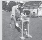
Flattener consists of a 20-ton jack mounted inside a heavy steel frame.
