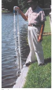
Simple emergency pump costs no more than \$25 to make, using materials that are easily obtained from any plumbing or hardware store.
