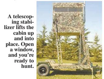
A telescoping stabilizer lifts the cabin up and into place. Open a window, and you’re ready to hunt.
