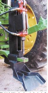
Hitch is held in place by a single pin. An 8-in. wide metal guide brings tongue into alignment.
