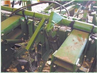
A single hydraulic cylinder rotates rockshaft to lift and lower the full rank of rolling shields at one time.
