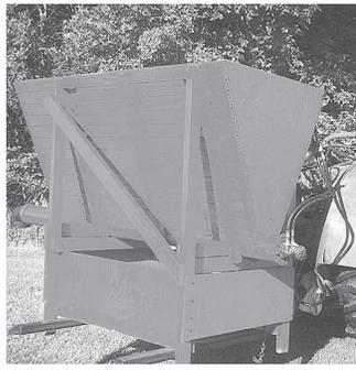
Power feed box holds 35 to 40 bu. of feed and rides on rear-mounted bale forks. An auger driven by an orbit motor extends several feet out from side of box.
