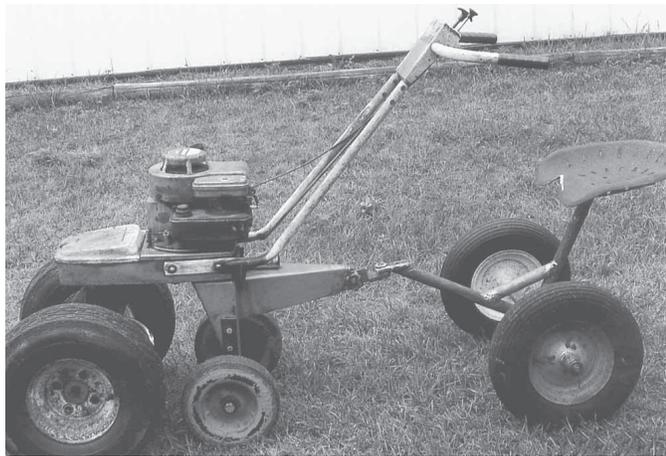
Home-built, 2-wheeled cart is powered by a Montgomery Wards walk-behind rototiller.
