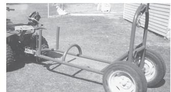
Hauler is made from steel tubing and is about 6 1/2 ft. long by 44 in. wide.
