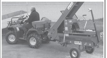
Two-wheeled firewood processor is equipped with a chainsaw cutting system, hydraulic splitter, and output conveyor.
