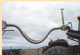
Exhaust is routed from the tractor muffler to a 14-ft. long, 2 by 2-ft. cooling chamber behind the tractor.
