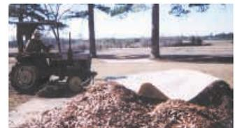
Pipe extends out right side of tractor and has a large piece of canvas attached to it that drags on the ground (left). Belly-mount mower on tractor blows leaves and grass clippings onto the canvas as it mows. Bryant drives to edge of yard and backs up to dump.
