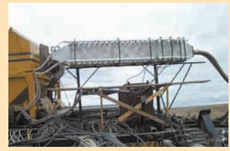
Air seeder's fan forces exhaust down through the same hoses that deliver seed and fertilizer to the ground.
