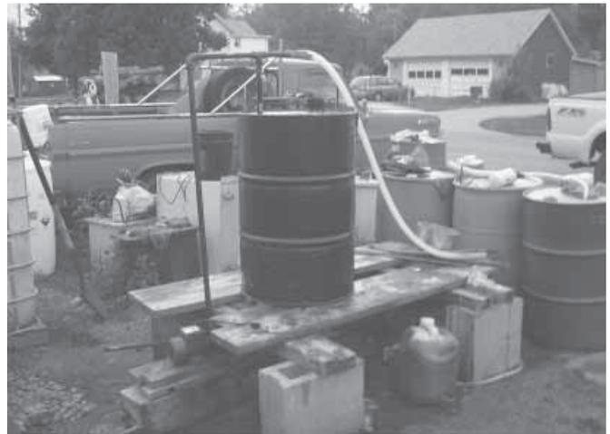
**Biodiesel processor is built from a steel 55-gal. barrel, an inexpensive pump, a black steel pipe, and brass valves.**
