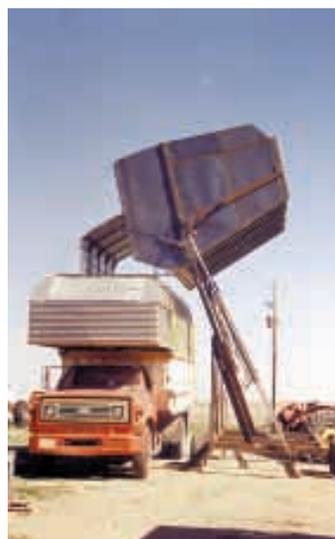
Wagon catches chaff and other fines while harvesting small grain, peas, canola and other crops. It's designed to lift and dump into a truck that's 15 ft. tall. Cantilever system automatically raises roof of wagon as bin tips to dump.
