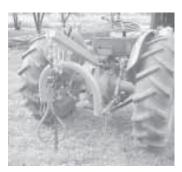
The 3-pt, log skidder has tongs that hook up to an adjustable-length chain, which attaches to one of three hooks on boom
