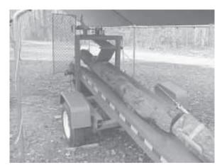
Winch pulls log onto splitting table where a chain saw is used to cut a 20-in. section.
