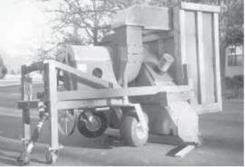
Larry Seiter turned an 18-in. dia. impeller vacuum that he obtained at work into a giant capacity, 3-pt. mounted, pto-operated leaf vacuum.
