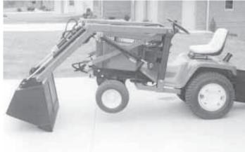
Using the "learn-as-you-go" method, Greg Lenz built this front-end loader for his Deere Loader is built strong enough to lift front end of tractor off the ground. 318 garden tractor.
