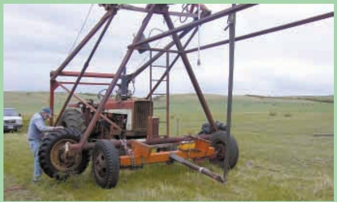
A loader tractor lifted each tower axle onto a saddle on top of a modified truck axle. Tower wheels were removed for transport.
