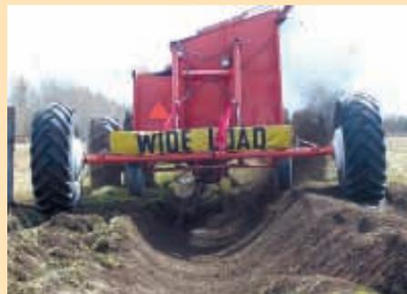
Machine makes ditches measuring 3 1/2 ft. deep by 7 ft. wide. Depth can be easily changed by shortening or lengthening chains on the cutter drum.
