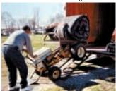
To operate the tractor, Lowe walks in front of machine and drives it backward. Operator can stand on fold-down front step to counter balance big loads.
