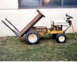
Dwayne Lowe turned a hydrostatic Cub Cadet into this walk-behind "mini forklift". It has a 30 by 48-in. dump bed with forks on front that tilt down for loading.
