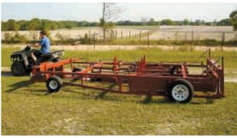
Lightweight, small square bale accumulator can be pulled behind an ATV, pickup, or small tractor.
