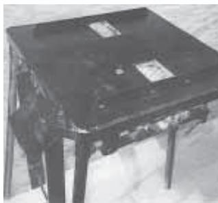
Simple in design, Carlson's brick-cleaning machine looks somewhat like a table saw. Dual cutting heads easily remove old, soft mortar from discarded bricks.
