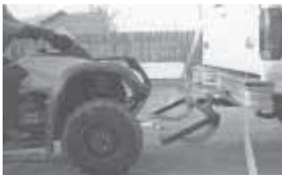
Front wheels are held by a cradle that fits into receiver hitch. The back end hangs free, supported by two 5,000-lb. nylon straps that run to the back of ATV.
