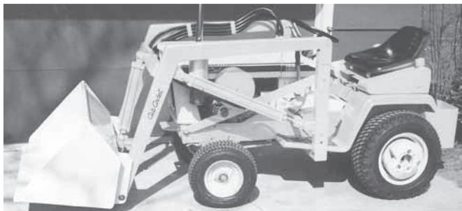
Belt-driven hydraulic pump and reservoir under hood provides lifting power. Three 1 by 2-in. hydraulic cylinders control loader - two to raise and lower the arms and one to tilt the bucket.
