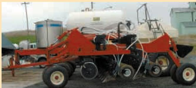
Three-section frame has one rank of coulters, two ranks of standards, a 130-bu. dual compartment seed fertilizer tank, and liquid fertilizer tanks.
