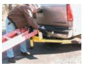
Ladder-holding attachment simply slips into receiver hitch.
