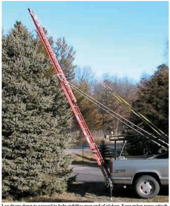
Leg drops down to ground to help stabilize rear end of pickup. Four nylon ropes attach to truck's stake box pockets.
