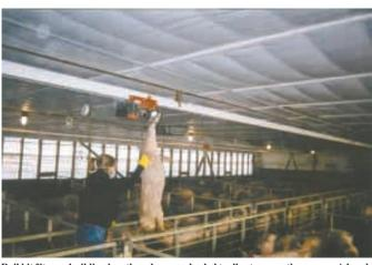
Rail kit fits any building length and uses a wheeled trolley to carry the carcass. A handheld control activates a 12-volt battery-operated hoist.
