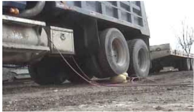
"Mightybag" works off a standard air compressor to lift loads up to 8,000 lbs.
