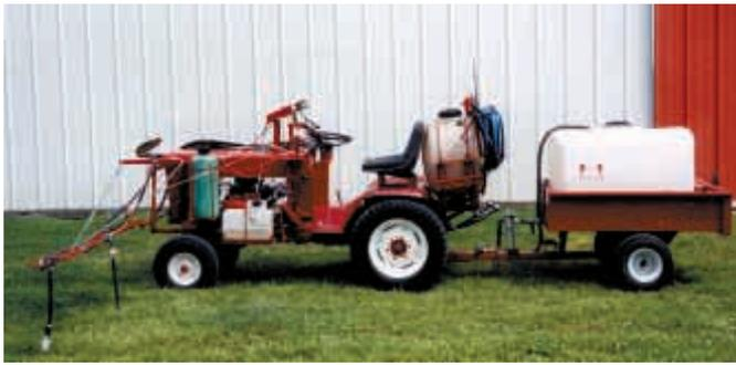
Gene Cafourek made this state-of-the-art self-propelled mini spray rig by mounting a 13 1/2-ft. boom on front of his 17 hp Bolens hydrostatic garden tractor.
