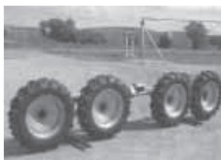
It's like putting dual wheels on a tractor except that the wheels run in-line, says the manufacturer.
