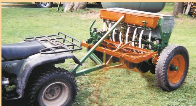
Zirbel cut his old 8-ft. Case drill into two 4-ft. plot drills, one for use with an ATV and one with a 3-pt. hitch for mounting on tractors.
