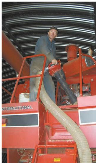
To keep chaff and grain dust off his combine, Phil Simrose uses a gas-powered leaf blower/vacuum with a 15-ft. section of hose clamped to it.
