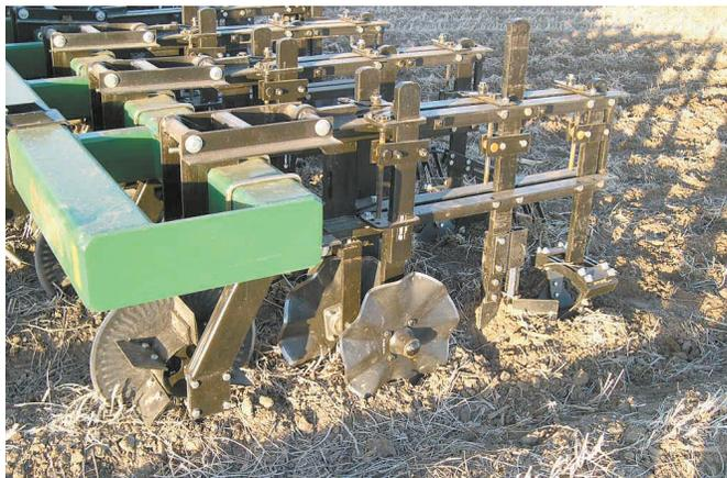
System consists of a 3-pt. mounted toolbar equipped with adjustable, clamp-on row units. Note chopping blade on up-front coulters.
